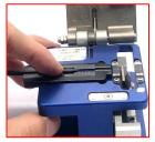
0.250mm Primary Coating: 20mm, 0.125mm Bare Fiber: 10 mm, total: 30mm ± 0.3mm
